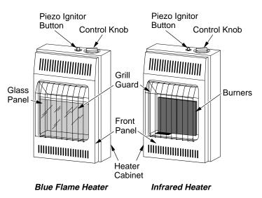
Figure 1 - Vent-Free Gas Heater
